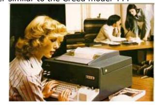
T150 This is a semi-electronic page printing teleprinter, with an electronic keyboard, operating at 50, 75 or 100 Bauds. The machine is powered by a 1400 rpm induction motor, but the timing is crystal controlled, and the machine is capable of operation at 45.45 Bauds by changing the crystal. As with the T100, the T150 is designed for single current operation only, and may be fitted with a punched tape reader and a tape punch. Internal signaling supplies are not usually fitted to this machine.
