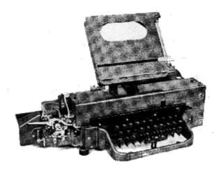
7P This is an off line keyboard perforator, introduced in 1934, whose sole function is to produce punched paper tape directly from the keyboard input. It may be found with either 1500 rpm governed or 1450 rpm induction motors. The punch mechanism is capable of working at up to 140
