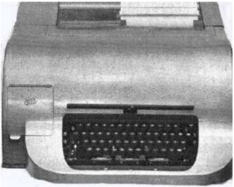
printing teleprinter was introduced in 1954 as a stop gap measure pending the development of a totally new teleprinter (the model 75), and is really only an advanced model 7E in an all enclosing silence cover. This makes it a very nice machine to
