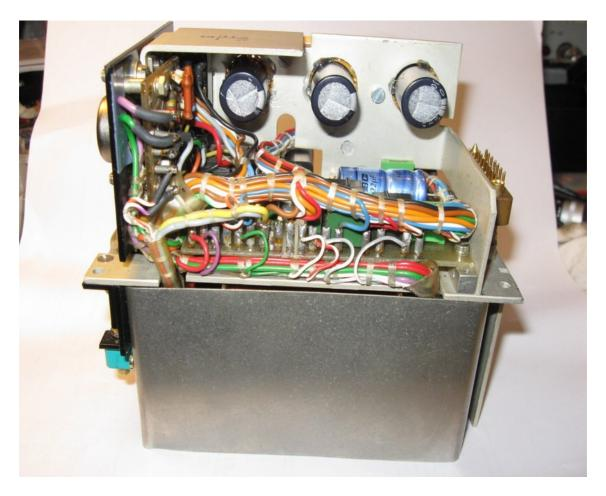
The unit is shown here reassembled. Note the placement of the new capacitors through the mounting holes of the old units.
